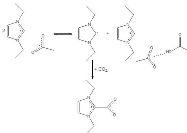
**Figure 5.** Proposed reaction mechanism for  $\text{CO}_2 + [\text{eem}][\text{Ac}]$  (i.e.,  $[\text{C}_2\text{C}_2\text{im}][\text{C}_1\text{CO}_2]$ ).<sup>105–108</sup>
