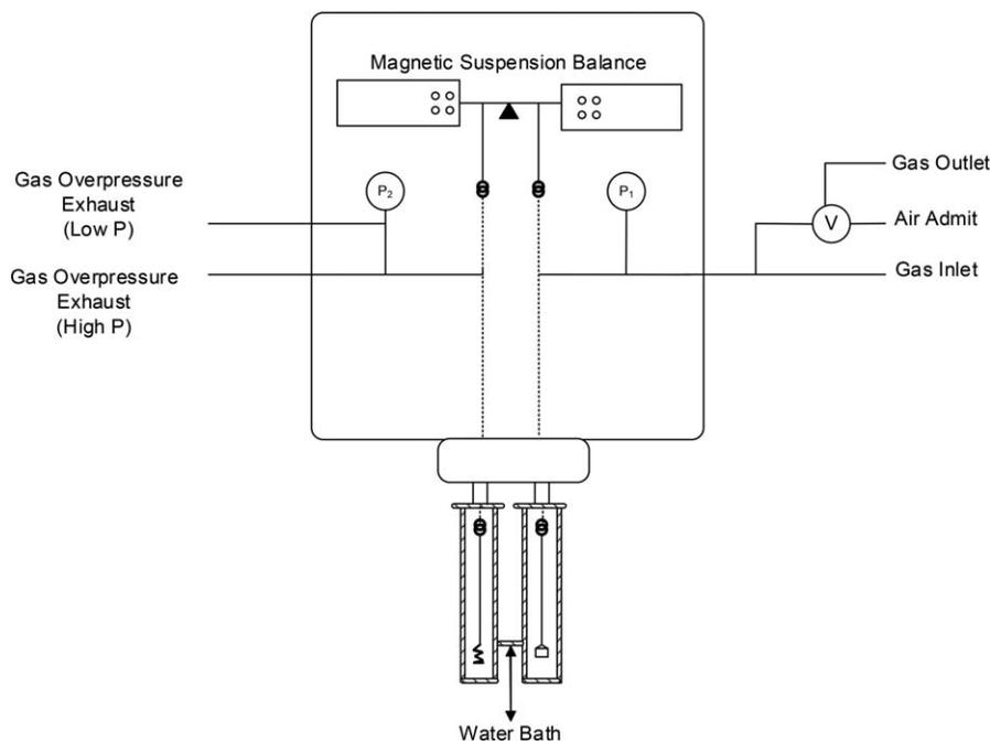
Figure 2. Schematic diagram of Hidden Isochema XEMIS gravimetric microbalance.<sup>54</sup>
