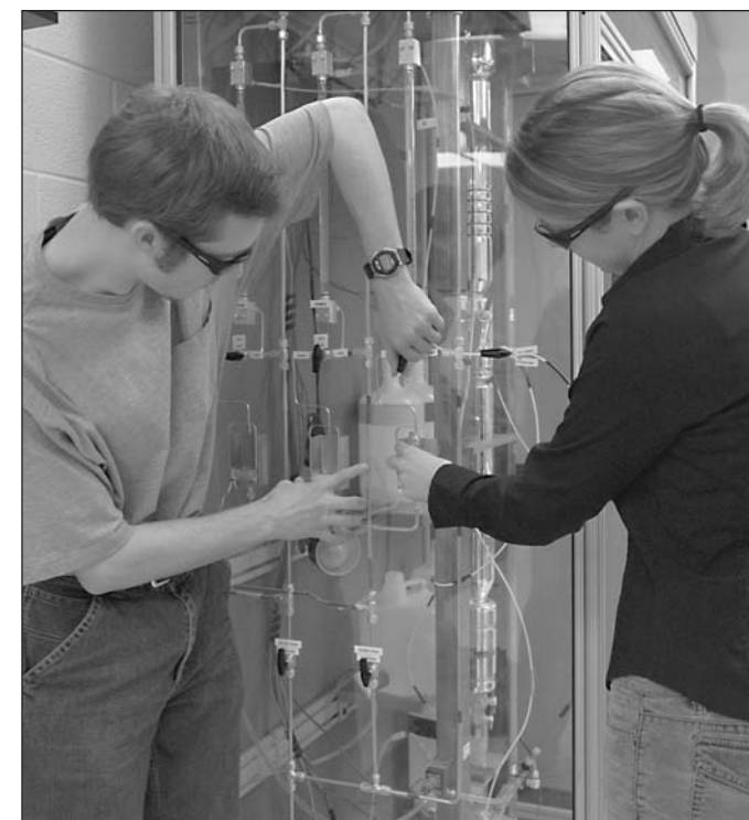
Two students operate the distillation column in the Chemical Engineering Unit Operations Laboratory.
